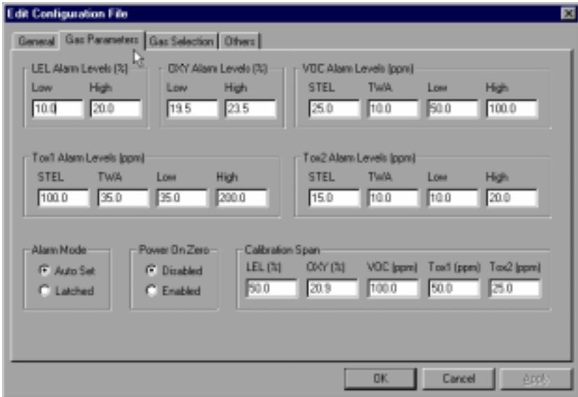
Figure 5-8 Gas Parameters Settings Tab Page LEL Alarm Levels (%): This is the place where the user can specify the low alarm level (%) and high alarm level (%) for LEL sensor.
