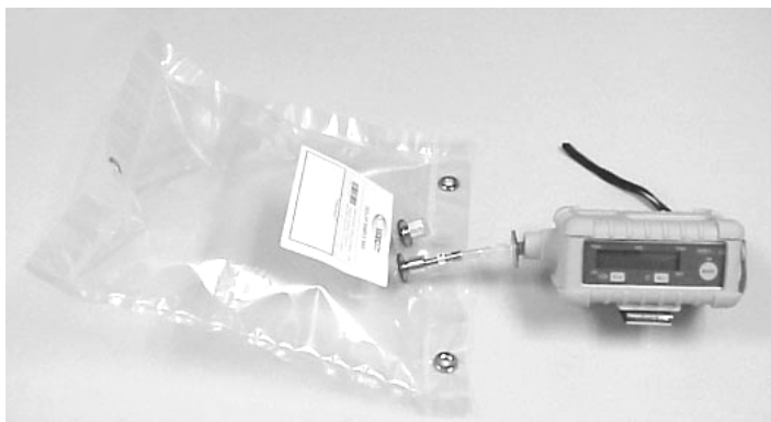
Figure 4-1 Connection of Calibration Gas
